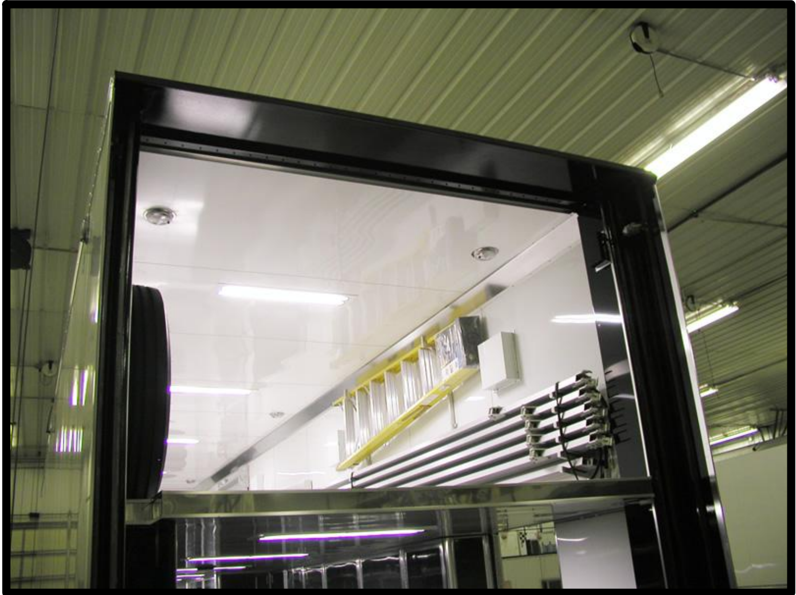
View of rear of trailer - attic level with awning pole and ladder storage
