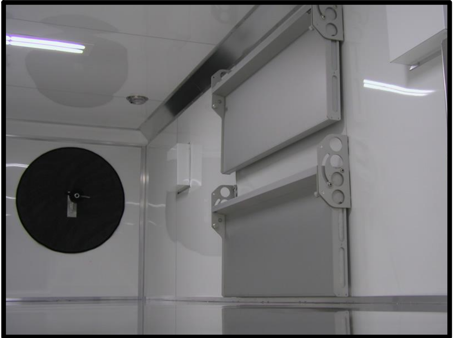
Upper level on the road side – wall mounted arrow flip bench/tables
