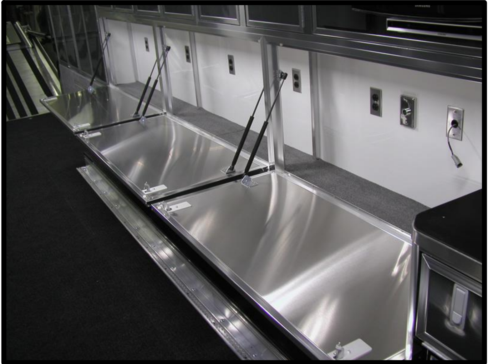
Cabinets on road side with large flip down doors - used as work surfaces
