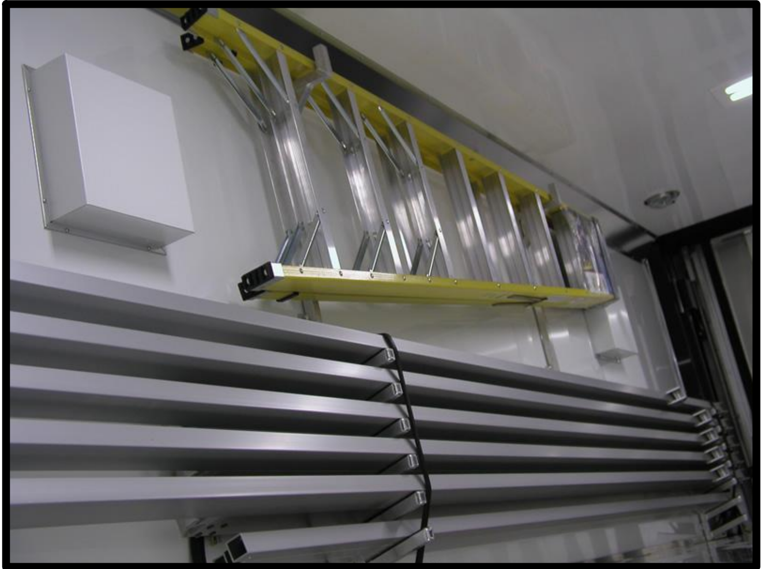
Upper level on curb side wall – ladder and awning pole storage
