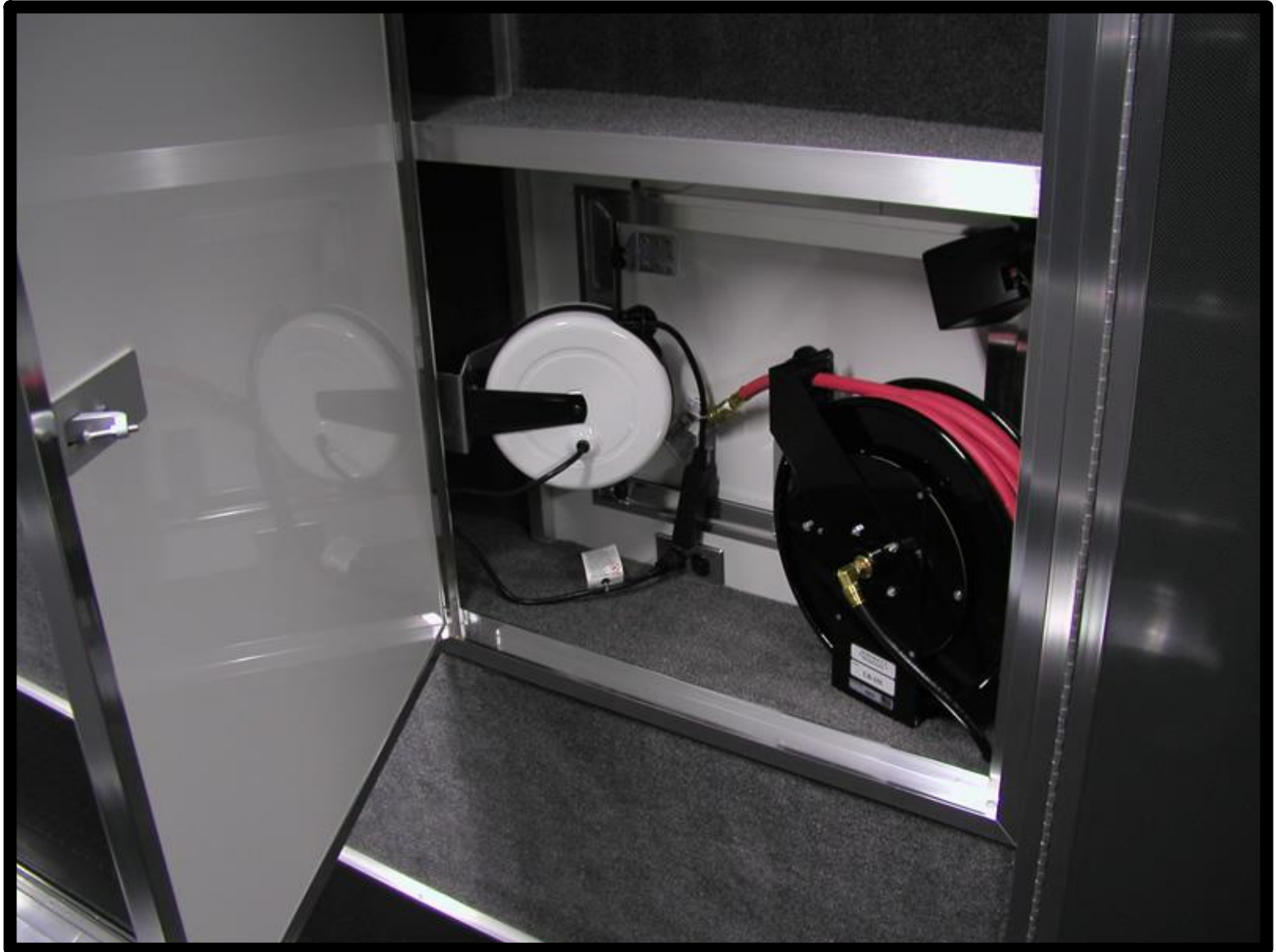
View of lower level work and storage area - air and electrical reels inside cabinet
