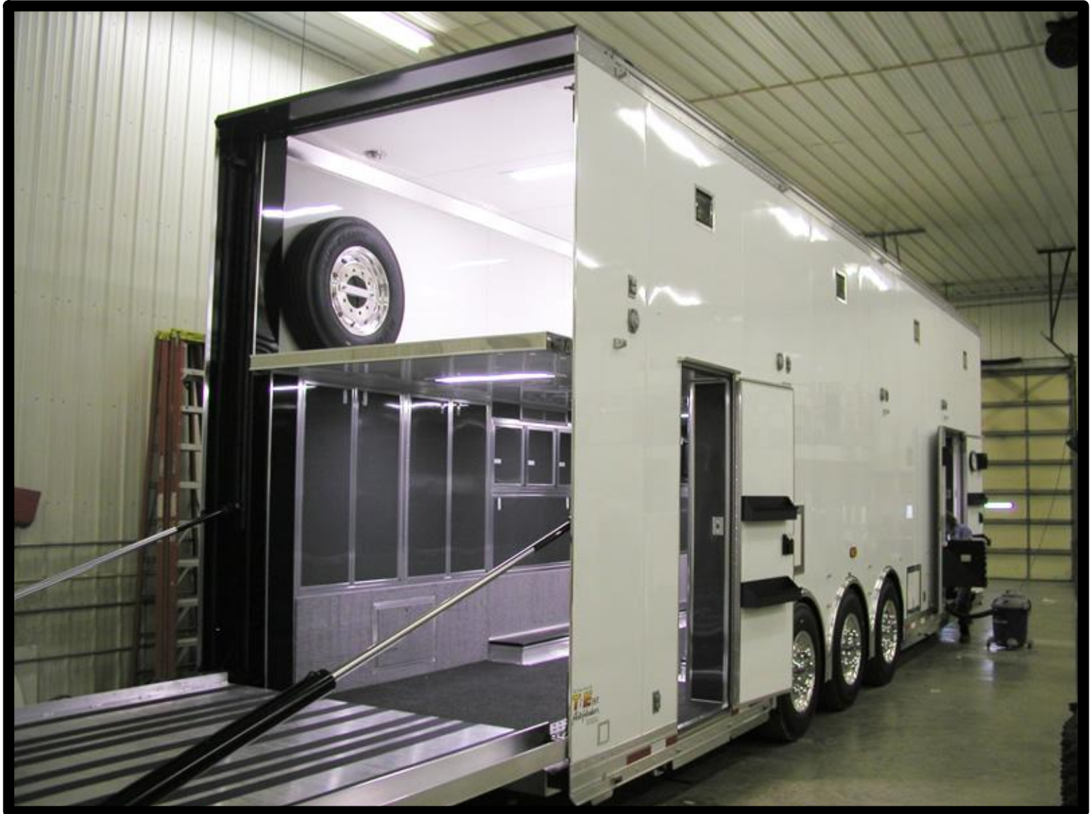
View of rear of trailer with lift gate in lowered position
