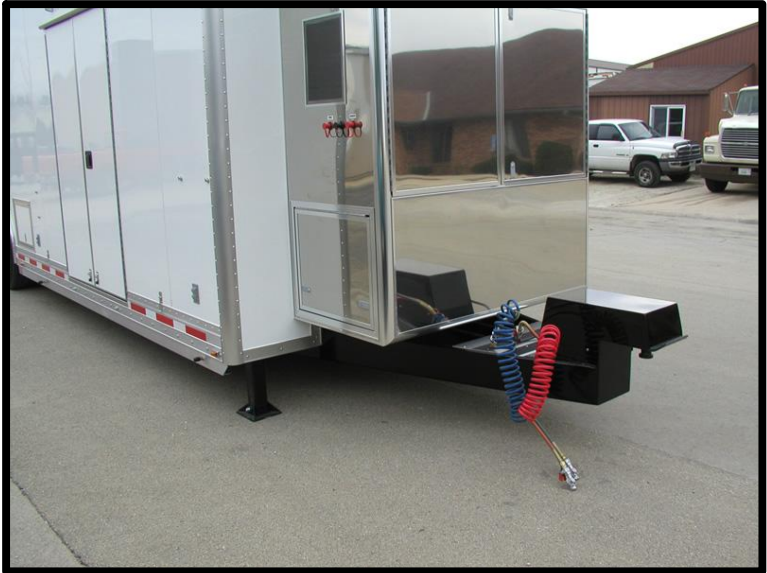
View of hitch and hydraulic landing legs
