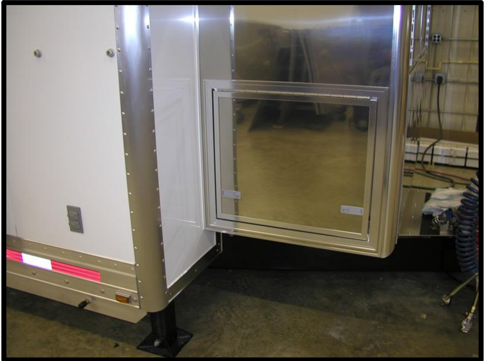
View of the front box assembly – door is over clutch grinder compartment
