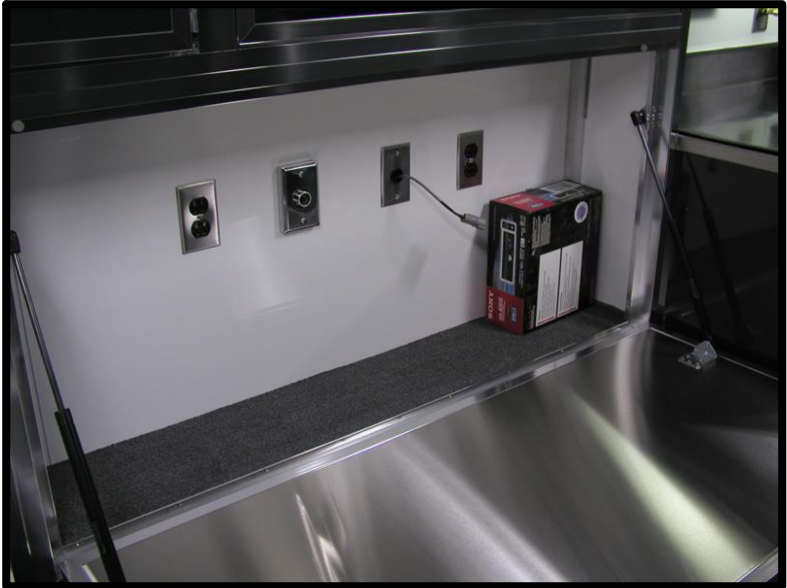
Cabinet on road side with large flip down door - used as work surface for PC station
