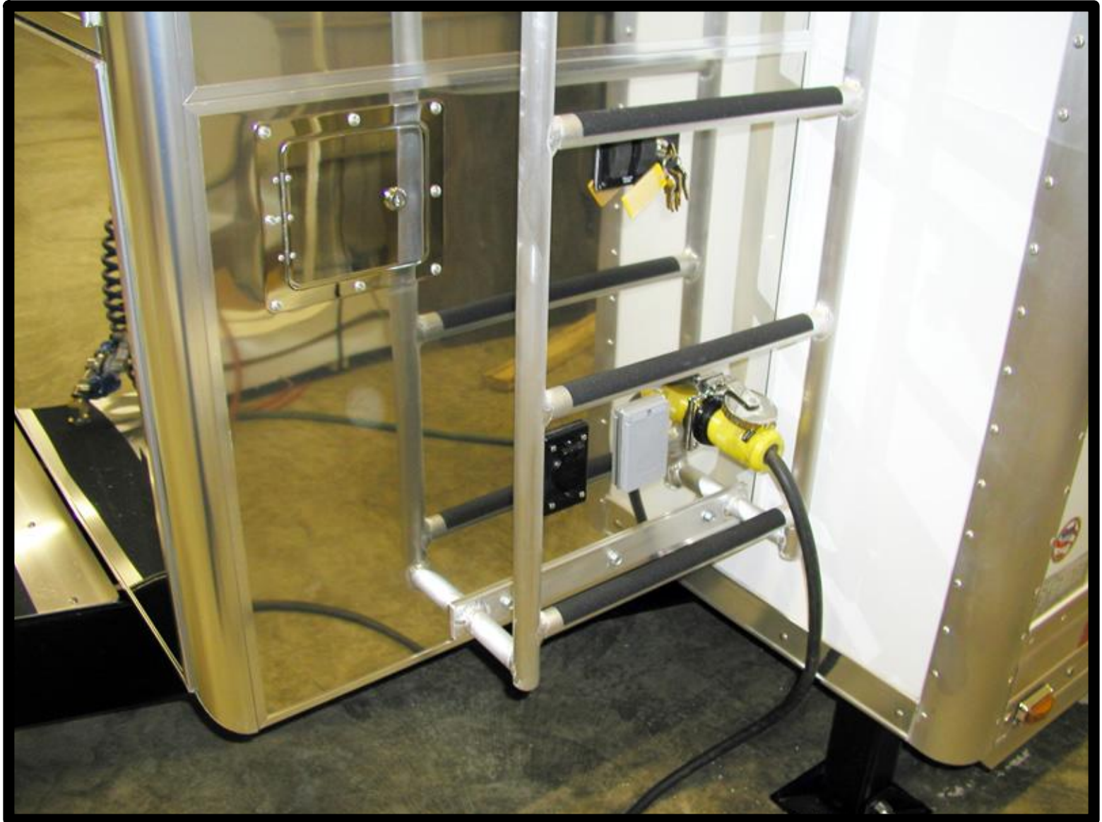
View of access ladder and power plug on curb side of front box assembly
