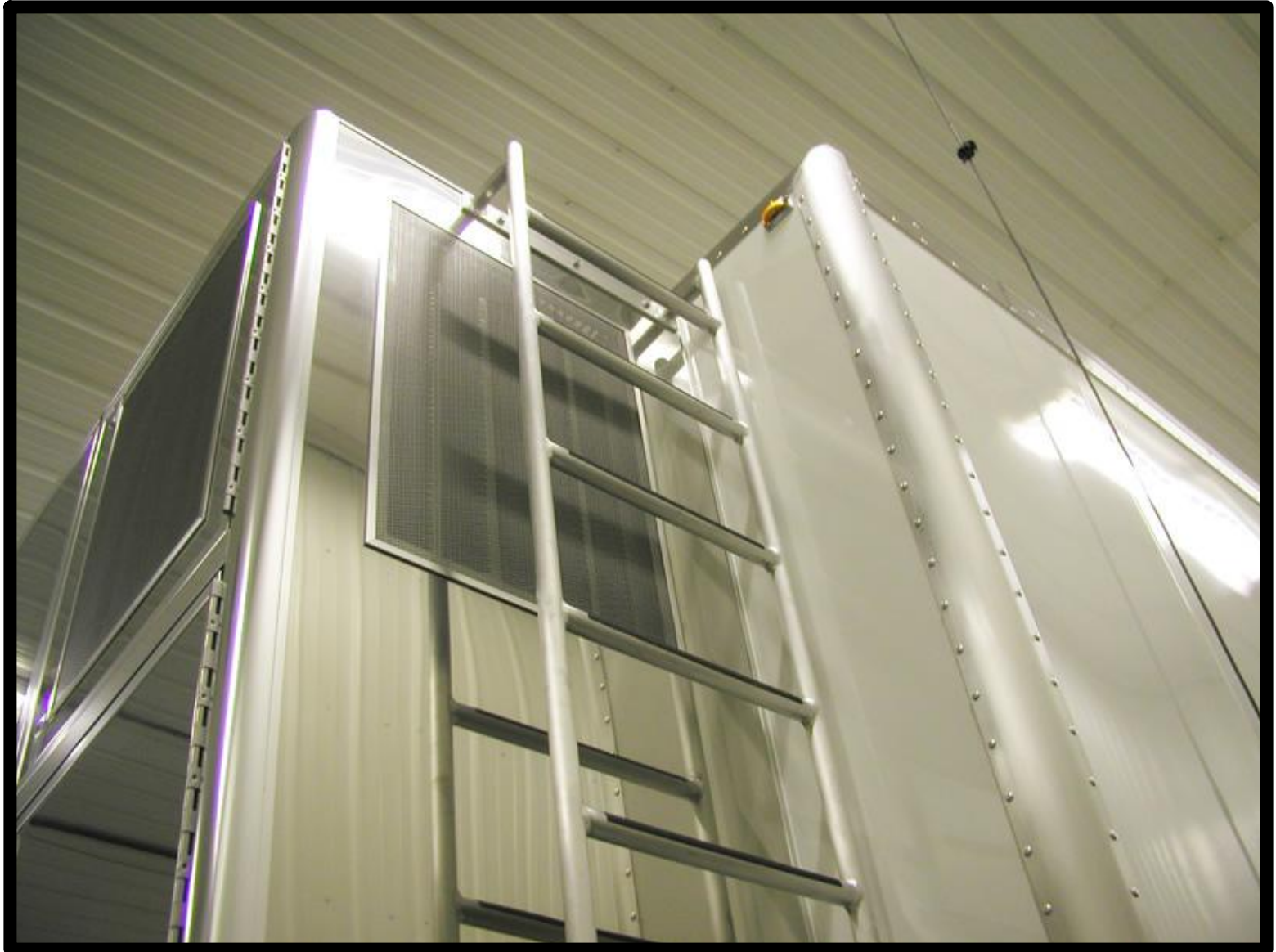
View of the top of the front box unit on curb side – A/C unit is behind screen
