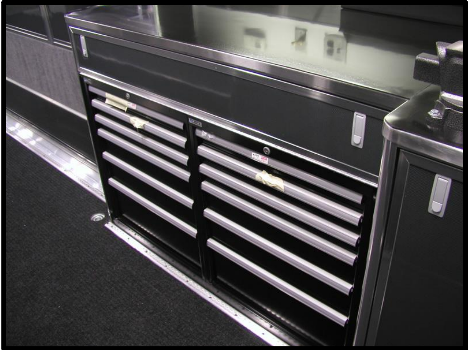
View of lower level work - dual Lista cabinets under work bench
