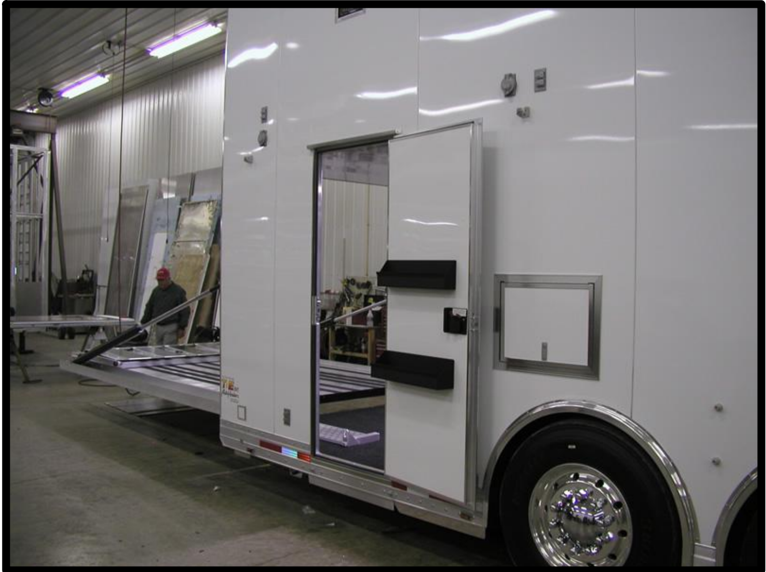
Rear side entry door w/trays – note air/electrical reel compartment above wheel well
