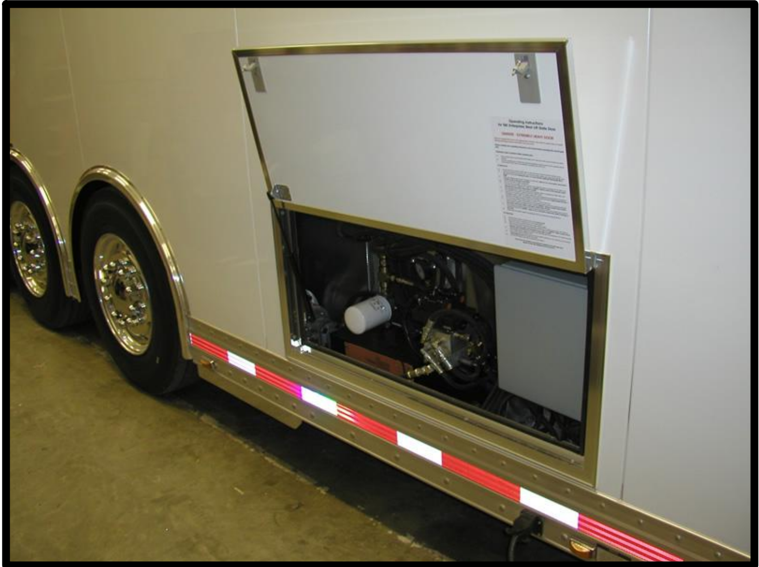
Lift gate hydraulics compartment on road side of trailer
