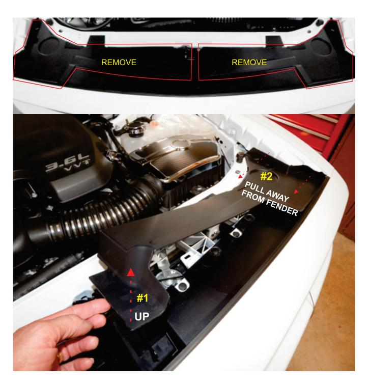
This is the view of the piece that ties into the radiator support from the upper portion of the front bumper cover. You will need to remove two of the three plastic tree inserts noted below on both sides of the bumper cover where it attaches to the radiator support. The ones closest to the fender on each side are not really sucking in the bumper cover so you don't need to worry about those.
