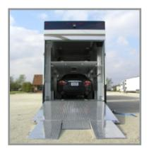
For T&E's standard type Pull-a-Long and Gooseneck trailers, we provide a heavy duty rear ramp door that can also be configured with optional beavertail extensions. For our smaller trailers this is probably quite suitable. We can provide optional electric winches to facilitate moving your vehicles into the trailer as well.
